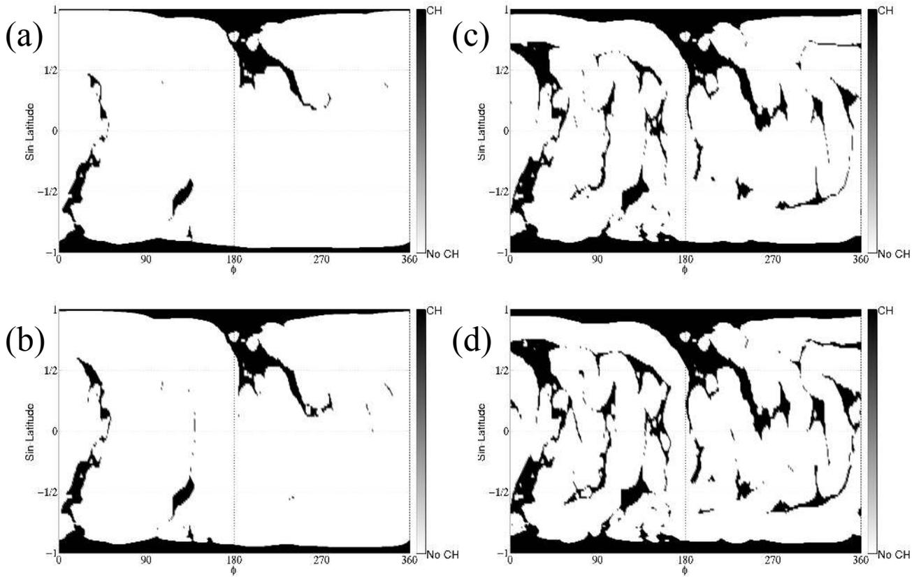
Fig. 2.— Open field regions (black) for four PFSS models using the NSO VSM CR2098 map for the boundary condition. (a)  $R_{SS} = 2.5R_S$ . (b)  $R_{SS} = 2.0R_S$ . (c)  $R_{SS} = 1.4R_S$ . (d)  $R_{SS} = 1.3R_S$ .
